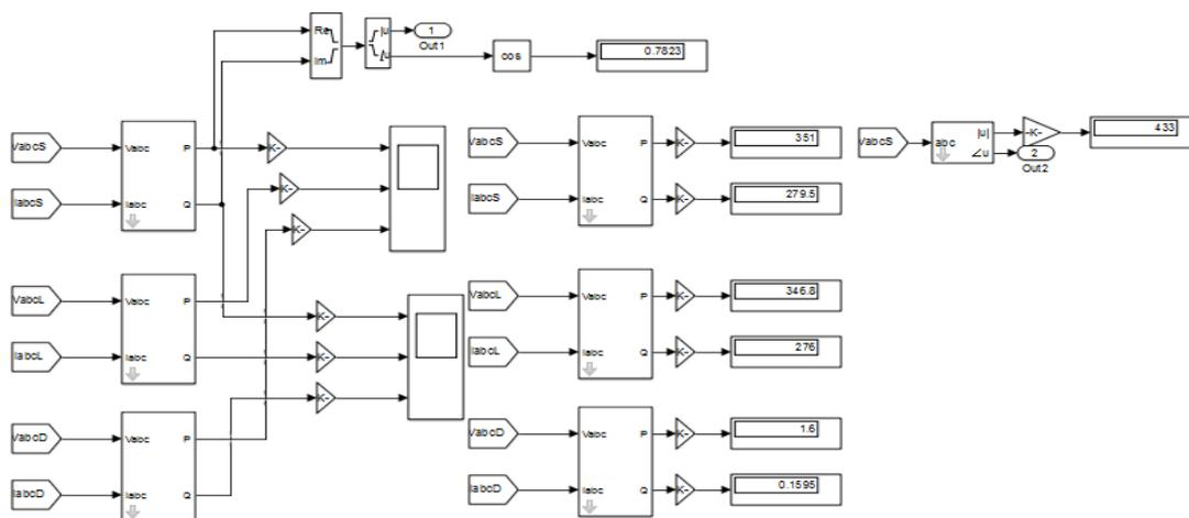
Figure 2 : Simulation model of transmission line with D-STATCOM
