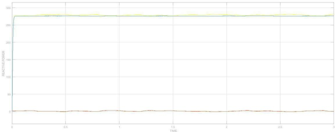
Figure 6 : Waveform of reactive power flow for source, load, D-STATCOM
