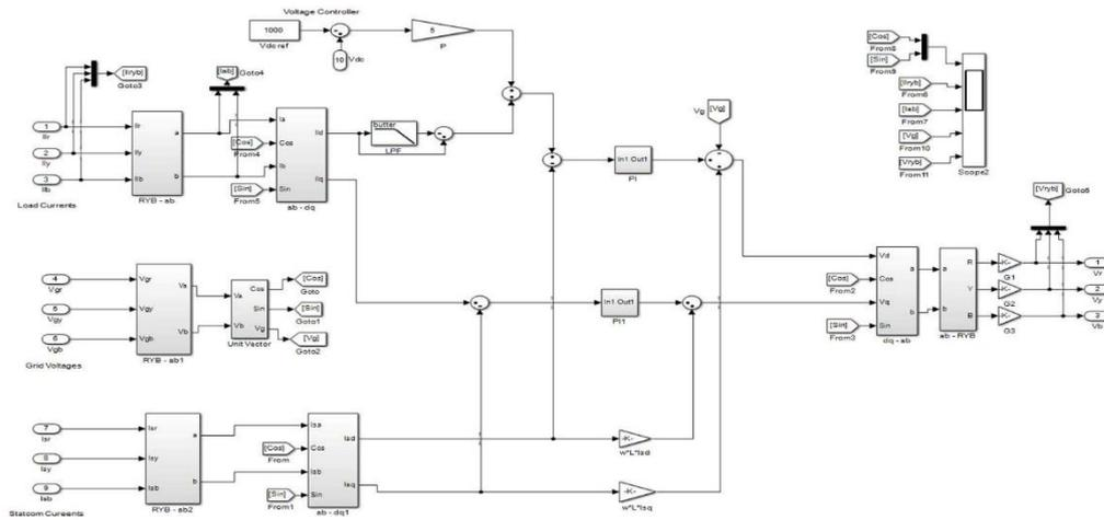
Figure 4 : Control circuit for VSI
