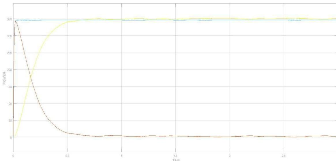
Figure 7 : Waveform of Real Power Flow for Source, Load, D-STATCOM
